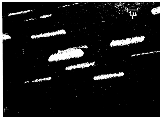
Fig. 2. The electron micrograph of the roof-like oxide formed on the cleavage surface of the stibnite.
